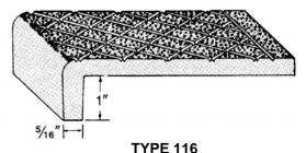
Standard nose - 1" Standard thickness - 5/16" Standard widths - 3", 4" and 6" DRAWING NOT TO SCALE
