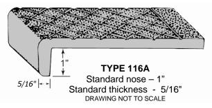
Can be furnished with a beveled back. Chief use superimposed on existing steps for repair and modernization. Also see Stairmaster series of extruded aluminum treads.
