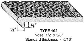
Standard widths - 3",4" and 6" DRAWING NOT TO SCALE
