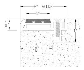
GUIDELINES FOR THE INSTALLATION OF METAL SAFETY TREADS OR NOSINGS INTO NEW CONCRETE OR STEEL PAN FILLED STAIRS: The use of very large aggregate in the concrete mix may make placement of the safety nosing difficult.
