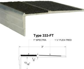
3" wide, 1/8" thick, nose 13/16" underside, 1" anti-slip filler strip in front, 1<sup>1</sup>/<sub>2</sub>" Flex-Tred® anti-slip tape in rear, beveled back
