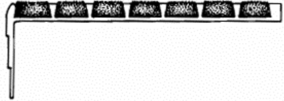
TYPE 142 4" wide, 1/4" thick, nose 1 1/8" underside DRAWING NOT TO SCALE
