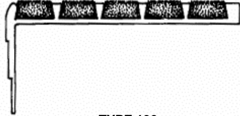
TYPE 132 3" wide, 1/4" thick, nose 1 1/8" underside DRAWING NOT TO SCALE
